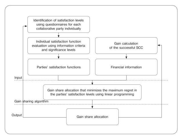
Fig. 1. The block diagram of the comprehensive gain sharing system
